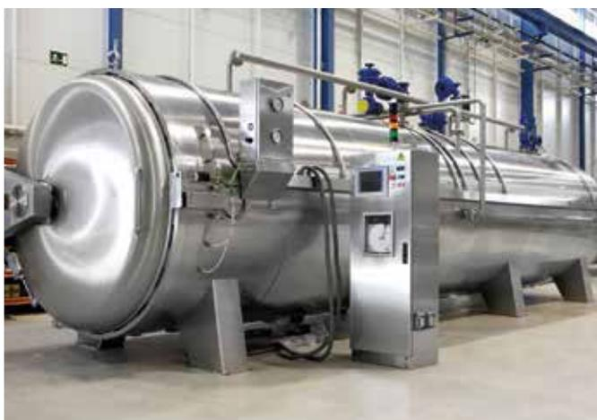
Designed for steam cooking tuna or similar fish, in a programmed manner, with vacuum pre-cooling (vacuum not forced by natural condensation of the interior vapour) and internal water showers.
